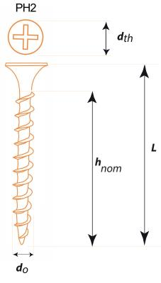
**The FFX Drywall Screw** with bugle head helps to prevent damage to the fixture surface. The single coarse thread allows smooth penetration into the base material. Its sharp point ensures easy take up into wood, chipboard and MDF.
